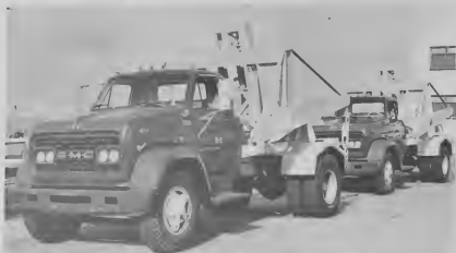
New modernized Dempster-Dumpster trucks have shorter body for better maneuverability in smaller areas.
